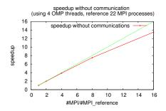
If we fit this curve to Amdahl's law  $\frac{1}{(1-p)+\frac{p}{x}}$  we get a non-parallel amount of 1.2%. This would result in a maximal MPI speedup of 83.
